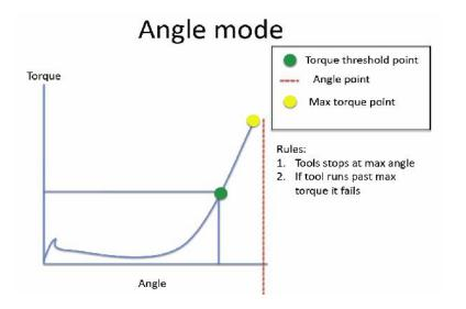
ANGLE/INPUT (A/IN): The threshold can't be set by the operator: in fact the value is the result of an external impulse through a proper contact (see paragraph "connections"). This function can be very useful if the operator wants the screw to rotate a certain number of
