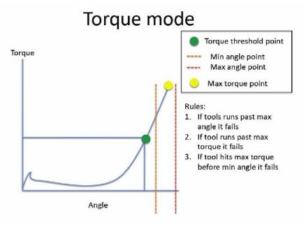
★ TORQUE/INPUT (T/IN): It corresponds to *Torque* mode, except for the threshold torque which can't be set by the operator: in fact the value is the result of an external impulse through a proper contact (see paragraph "connections"). It can be very useful if the operator wants the control unit to start counting the angle from a position which is indicated by a precision instrument.
