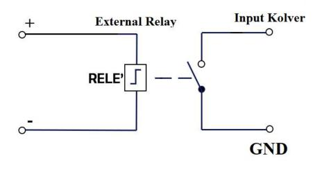
As for the outputs, they are all PNP type with active function. On each pin you will have 24V DC. Control unit Output
