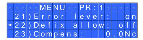
**21**) **Error lever:** when ON, an error signal will occur when the lever has released before reaching the torque.
