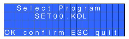
2) Write USB: press OK and create your new SETxx.KOL application where you save all the parameters you have set in the control unit.
